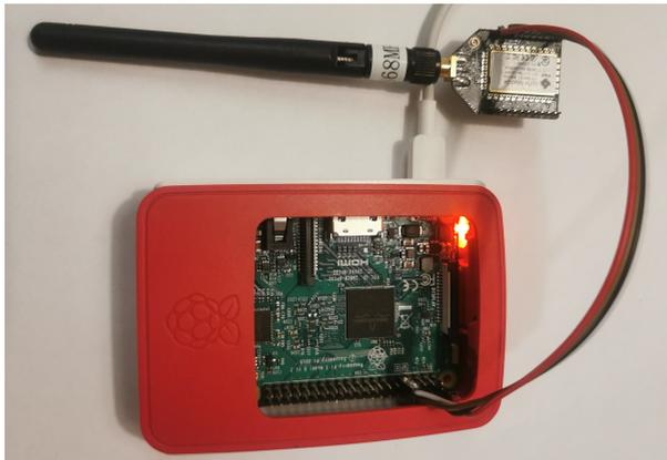
**Figure 10.10:** Picture of the hardware used as the central node: RaspberryPi 3B with a RAK811 LoRa module connected over Serial.
