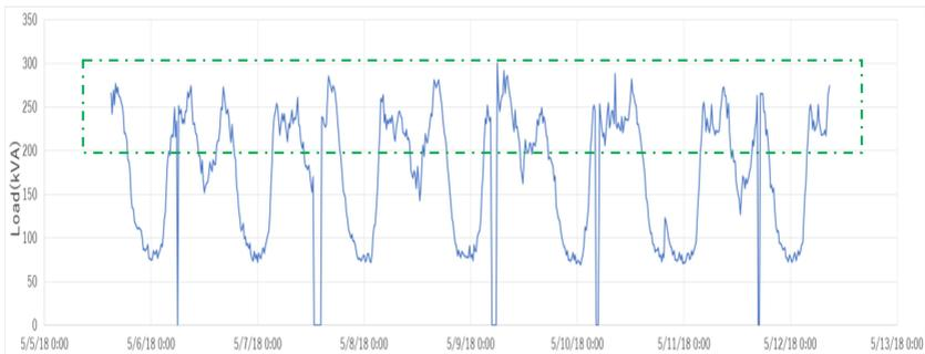
**Figure 2.7:** An example of transformer loading measurement result (Transformer rated capacity: 200kVA).
