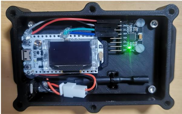
**Figure 10.12:** Picture of the real sensor node without assembled top part of the case.
