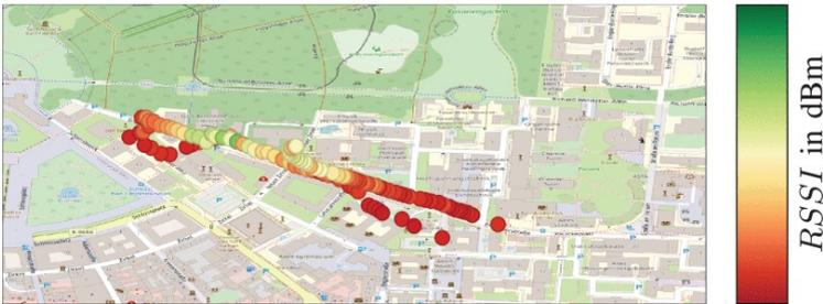
**Figure 10.13:** Range testing for  $SF = 7$  using a GPS module in combination with the Heltec node, color coding the RSSI the packet was received with.
