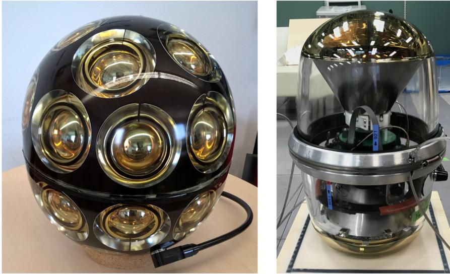
Figure 3.13: Prototype of mDOM and D-Egg. These will be tested in IceCube-Upgrade[230]. PC: IColl.
