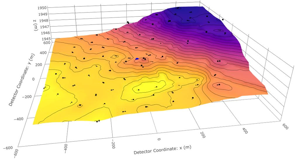
Figure 3.7: Height variation among IT tanks (black-dots), without snow coverage. Inverse Distance Interpolation [170] is used to estimate the IT-surface (from the sparse measurements at IT-tank location), and the contours. ICL is denoted by the blue-circle in the center.
