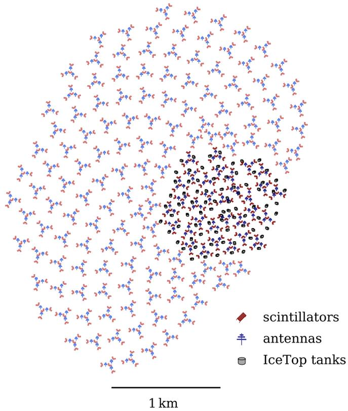
Figure 3.15: Planned layout of the Surface-Array component of IceCube-Gen2 Observatory, with the current IceTop Array. The surface array will constitute multiple stations, each constituting 8 scintillation detectors and 3 radio antennas. Plot from [243].
