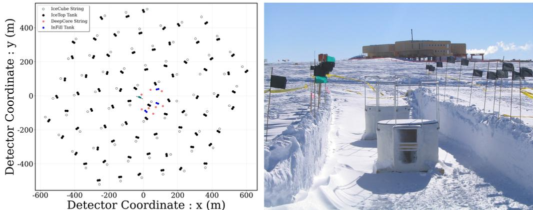
Figure 3.6: **Left:** A schematic of IceTop array. The **IC** strings, **DC** strings, and **ICL**(sea-green colored structure in the middle) locations are also depicted. **Right:** An IceTop station consisting of two ice-Cherenkov tanks, during deployment. **PC:** **IColl**.
