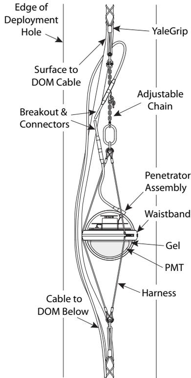
Figure 3.4: DOM on an in-ice cable. Illustration from [163].
