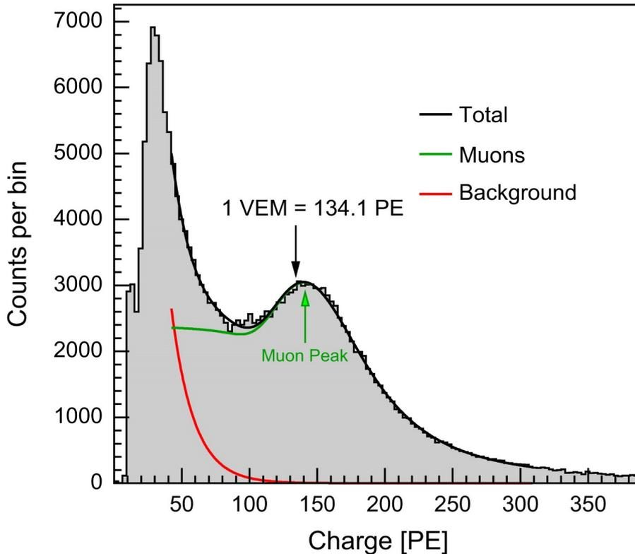
Figure 3.12: Charge spectrum at [HG-DOM](#) in tank 61A at [IT](#), and fit to obtain [EM](#) and muonic component. 1 [VEM](#) = 95% of muonic peak-value. Plot borrowed from [\[202\]](#).
