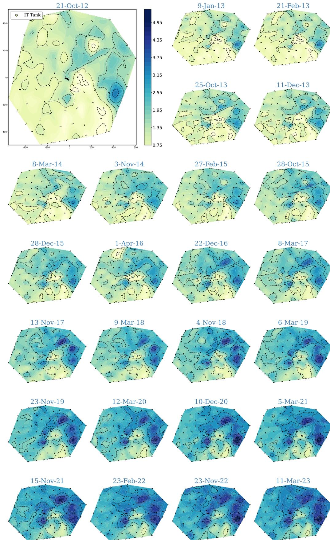
Figure 3.8: Change in snow-accumulation on IT-tanks over multiple years. IT is considered as a plane surface here.
