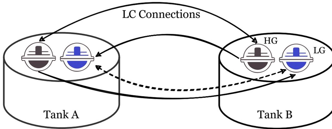
Figure 3.11: Cabling done to check LC at an IT station. Each IT station consists of two tanks with two DOMs each (high-gain = HG and low-gain = LG). The connection between the LG-DOMs is only used if the HG-DOM dies.
