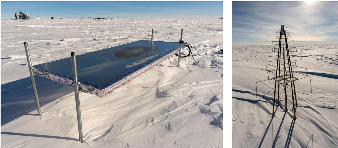
Figure 3.16: Elevated scintillator-panel (left) and radio-antenna (right) at the South-Pole. PC: IColl.
