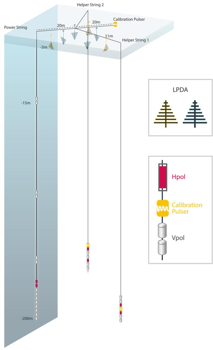
Figure 3.17: Hybrid radio station for the planned extended radio array. Picture from [244].
