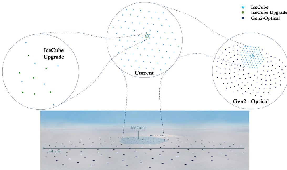
Figure 3.14: Planned design (*Top View*) of the extended IceCube-Gen2 optical component (*right: Dark-Blue Dots*) with the current IceCube Array (*center: Light-Blue Stars*) with the planned seven low-energy IceCube Upgrade strings (*left: Green Dots*). The extended radio array (not shown here) extends farther beyond the planned IceCube-Gen2 Observatory.
