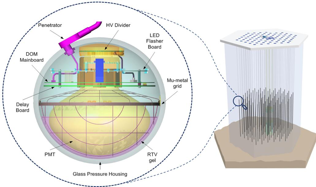
Figure 3.3: Schematic of Digital Optical Modules (DOMs) used at ICNO.
