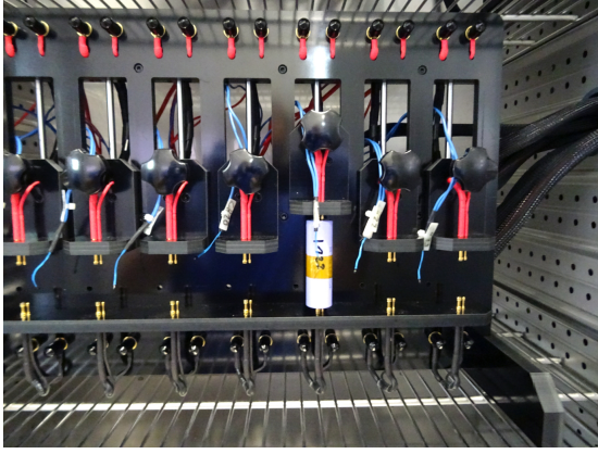
Fig. 2. An inside view of the climate chamber: A single cell connected to the battery cycler.
