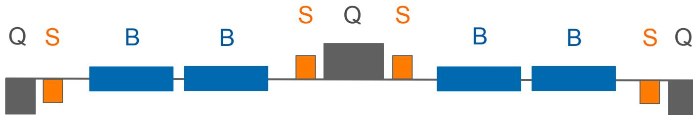
B = bending magnet, Q = quadrupole, S = sextupole
