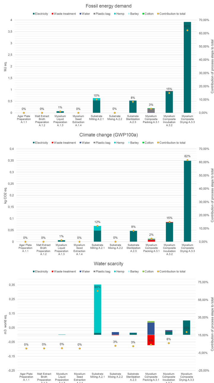
Fig. 3. LCIA results for fossil energy demand, climate change, and water scarcity for the production of 1 kg of hemp-based MBC (according to impact assessment methods listed in Table 3 and results listed in Table 4).
