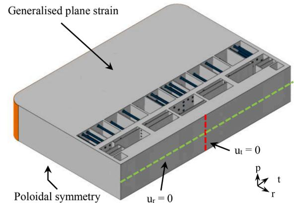
Fig. 6. The mechanical restraints [11].
