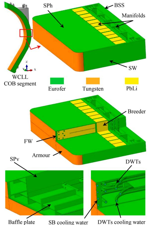
Fig. 2. Geometric model of the WCLL COB equatorial region.
