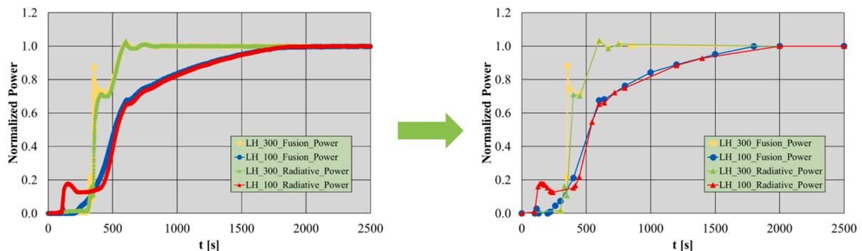
Fig. 1. Time evolution of fusion power  $P_{fus}$  and radiative power  $P_{rad}$  calculated with ASTRA for the cases with L-H transition at  $t = 100$  s and  $t = 300$  s. The left plot shows the original ASTRA results, while the right plot highlights the points employed for the thermomechanical analysis.
