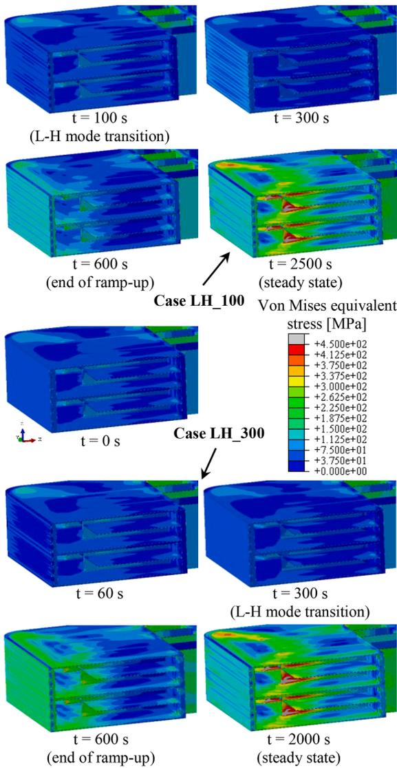
Fig. 7. Equivalent Von Mises stress field – section view.
