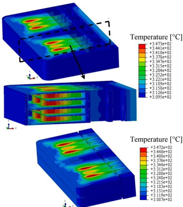
Fig. 3. The temperature initial condition.
