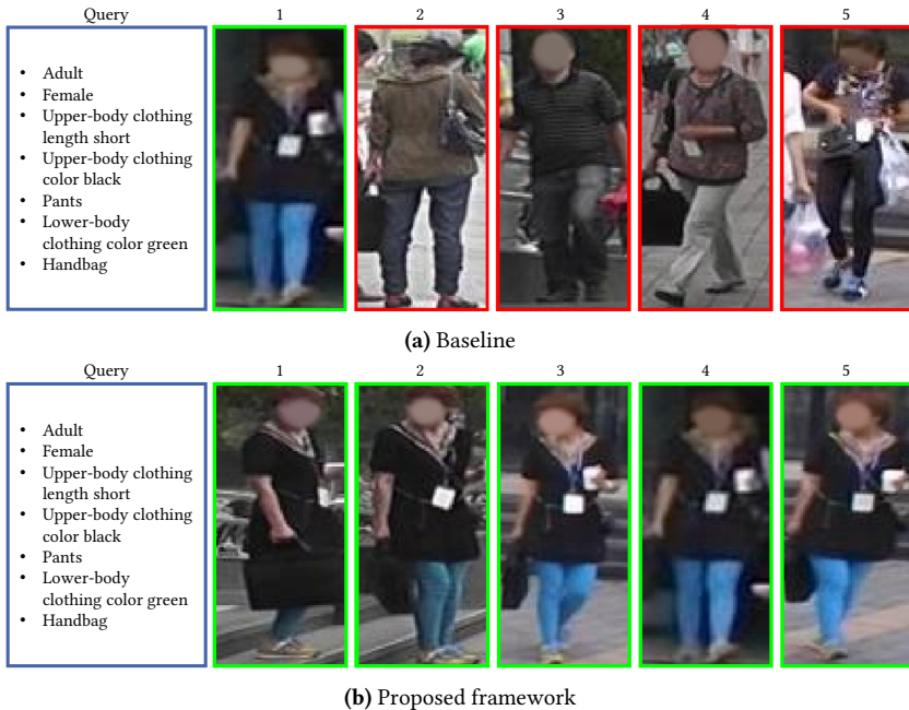
Figure 8.2: First qualitative specialization result – In contrast to the baseline approach, the proposed framework retrieves five matching images. The figure shows an example for the Market-1501 [Zhe15, Lin19] dataset. The blue boxes include the query attributes and green and red borders stand for correctly retrieved images and images deviating from the query, respectively.
