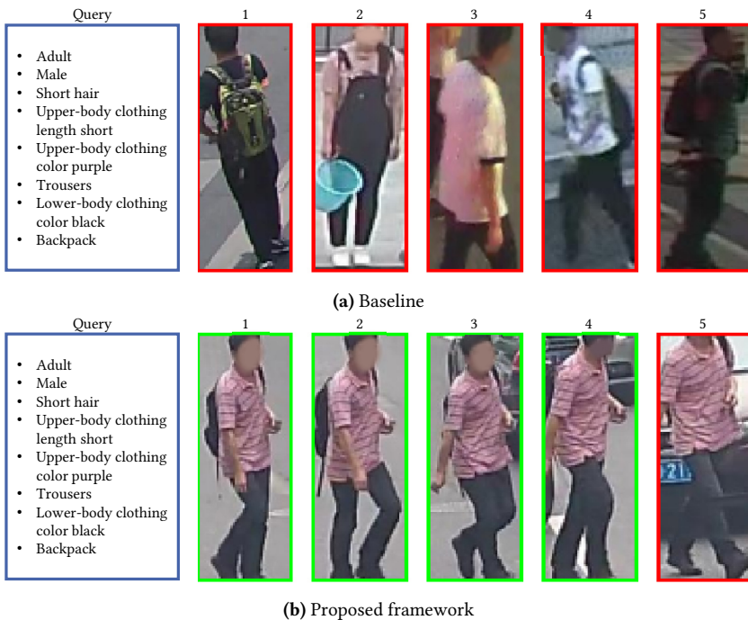
Figure 8.6: Second qualitative generalization result – The figure shows a generalization example from the UPAR dataset. The blue boxes include the query attributes and green and red borders stand for correctly retrieved images and images deviating from the query, respectively. The proposed framework is able to retrieve gallery samples at early ranking positions even when relevant attributes, such as the backpack, are invisible. Source of the images: [Liu17].
