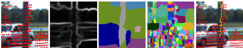
Figure 3.3: Semantic aware geodesic distance. Given an input image the pixel-wise edge costs and semantics are calculated. The edge and semantic cues are combined to calculate a geodesic distance between each pixel. The approximation in Section 3.3.3 assigns to their geodesic closest measurement resulting in Voronoi cells. The geodesic distance is then used to determine a graph that connects semantically related measurements (the yellow line on the right image shows the 20 closest measurements to the measurement selected in green). Adapted from [101].
