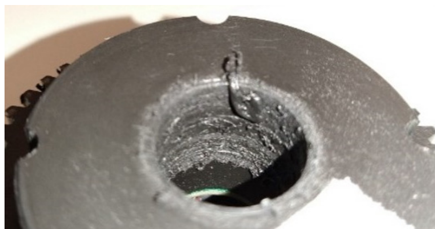
Figure 4. Molten shaft hub connection of gear 2 after failure.
