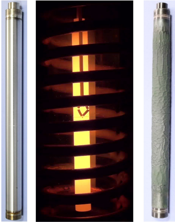
Fig. 6 Cr-coated samples before (left), during (mid), and after transient experiment at up to > 1500\text{ }^{\circ}\text{C}
