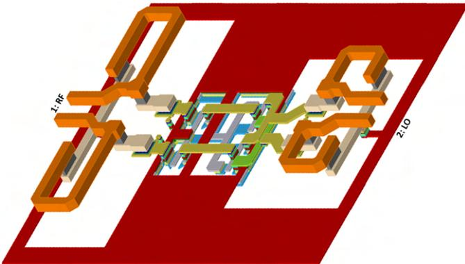
Figure 3.7: 3D layout view taken from EM simulation setup of the down-conversion mixer.
