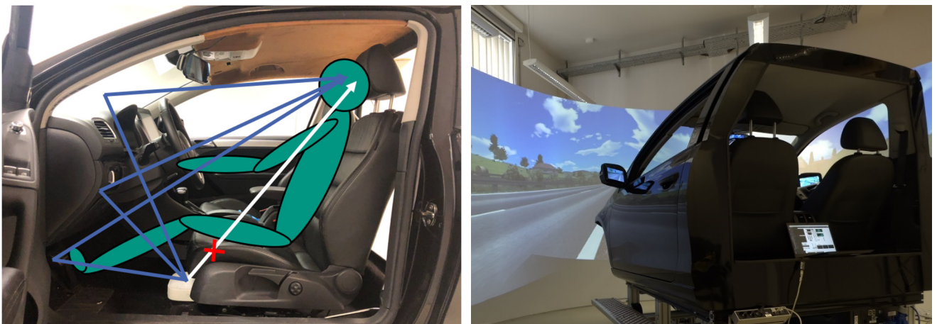
Figure 4 (Left Figure). Transfer paths from Speaker to driver ear. Interrupted direct transfer path in white, and transfer paths via reflected sound waves in blue. (Right Figure). Open back side of the vehicle cabin in the driving simulator.
