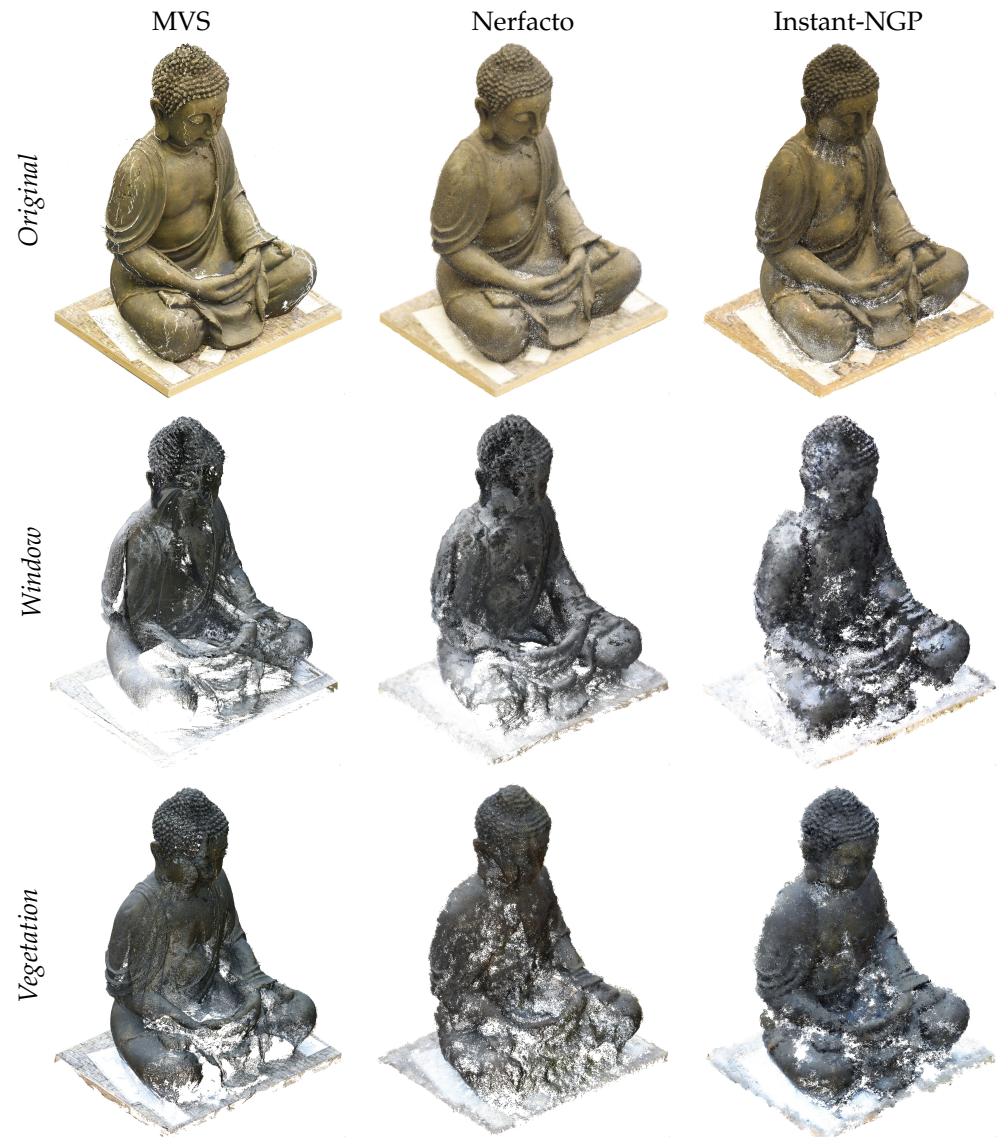
Figure 5. Qualitative comparison of the point cloud geometric reconstructions for all used methods: MVS, Nerfacto and Instant-NGP in all scenarios: without obstacles, occlusions and visibility constraints ( Original ), transparent ( Window ) and non-transparent ( Vegetation ) obstacles respectively. MVS shows gaps in reconstructing the geometry of the occluded parts, while NeRFs exhibit in completeness.
