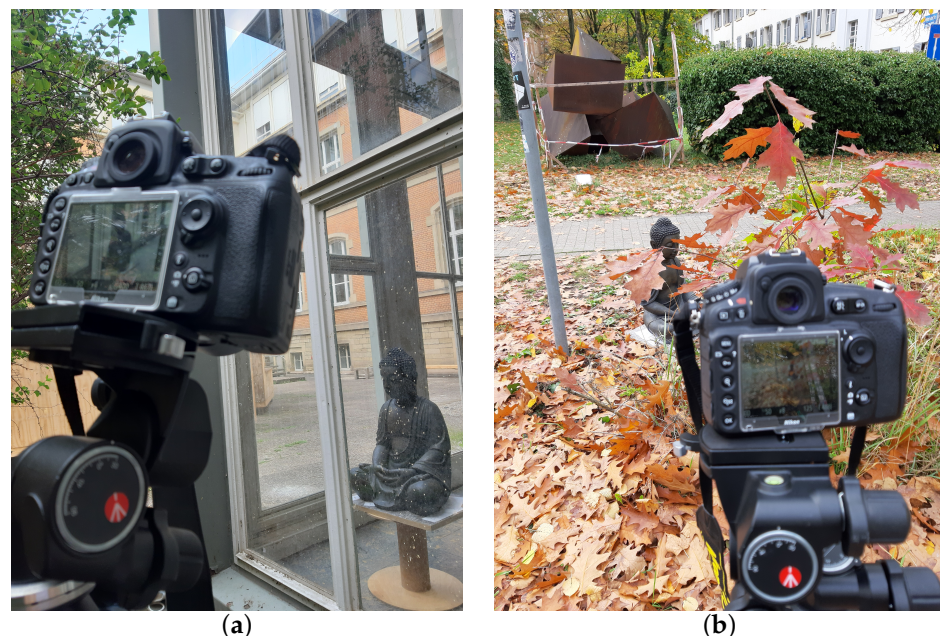
Figure 2. Image capturing setup for both obstacle scenarios with Nikon D810 SLR mounted on a tripod: (a) We place the object behind windows whose glass isn't completely transparent, it has dust and paint dots which make the reconstruction challenging; (b) Different vegetation coverage is considered in the front side of the object.
