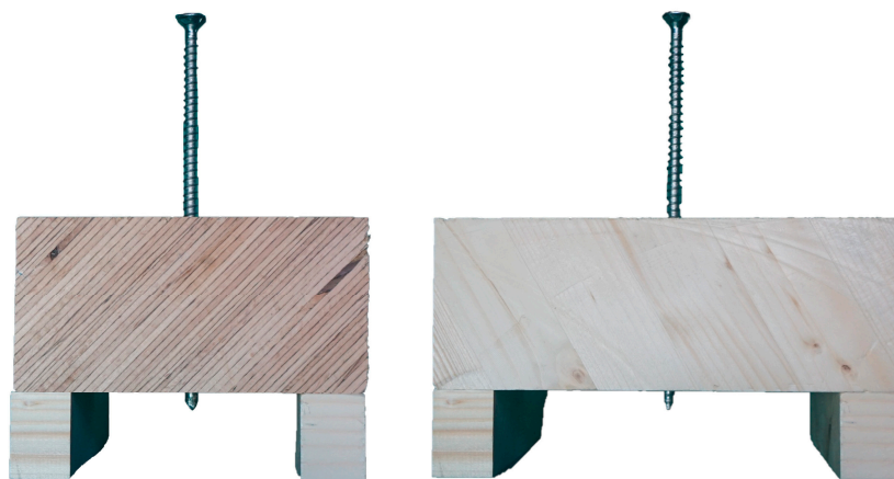
Figure 1. Timber products tested: beech-LVL (left) and GLT from spruce ( Picea albies ) (right) with different load-to grain angles (45° (left) and 30° (right)).
