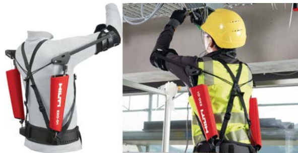
Fig. 1. The "EXO-O1 Overhead Exoskeleton" manufactured by Hilti serves as an example of the Passive Upper Limb Exoskeleton (ULE) and the industrial application of exoskeletons. Here, the lack of sensors, electronics and motors is evident, as the system solely relies on the energy stored in its elastic binders to generate an upward force on the component connected to the elbows. Illustrations retrieved from [12].
