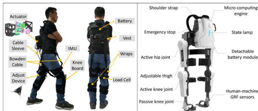
Fig. 2. The image comprises two illustrations of lower limb exoskeletons: (a) depicts a soft LLE. This exoskeleton introduces a soft system design. The Bowden cable generates tensile force and torque for movement, while load cells measure force and the IMU (Inertial Measurement Unit) sensor collects orientation, velocity, and acceleration data, enhancing control and response. Retrieved from [32]. (b) showcases a rigid LLE, UGO. This exoskeleton aids balanced walking for patients with spinal cord injuries or stroke. It features powered hip and knee joints and a passive ankle joint. Sensors and encoders provide data on joint angle and torque. Retrieved from [33].
