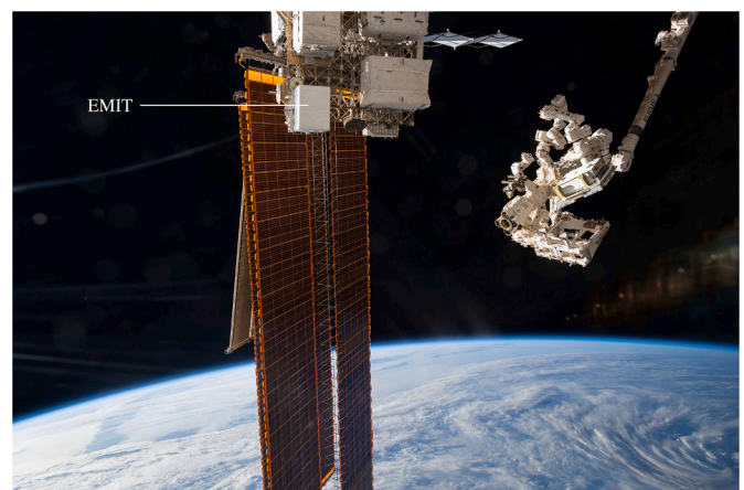
Fig. 1. EMIT deployed to the ISS. EMIT is the white box mounted at the lower left on the ELC1 rack at the top of the image. Credit: NASA.
