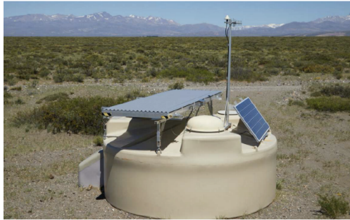
Figure 2.2: The water Cherenkov detector station of the surface detector. Left: Photograph of the WCD station. Figure from [112]. Right: Schematic view of one WCD station. Figure from [113]. A detailed description of the design and operation of the WCD can be found in the text.
