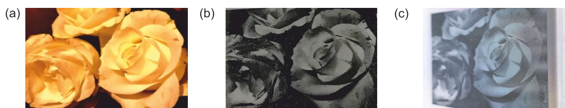
Figure 7.14: Fabricated smart window with a pixelated and high dynamic range of haze. (a) The original rose image used. (b) Fabricated smart window with a well-replicated rose image in a released state. (c) The fabricated smart window at a large viewing angle preserving a good displaying quality.
