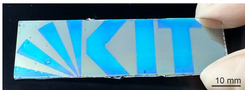
Figure 6.17: Inkjet-printed patterned filter.
