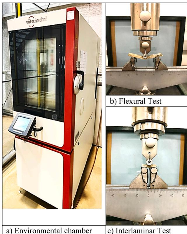
Fig. 2. : Aging and mechanical tests for hybrid composites.
