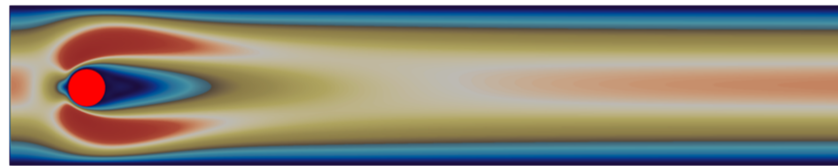
(a) Example of the 2D cylinder from OpenLB with Re = 20 .
