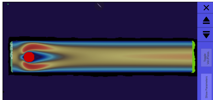
(b) Simulation of a hand-drawn domain using paint2sim with Re = 20 replicating the example used for validation.
