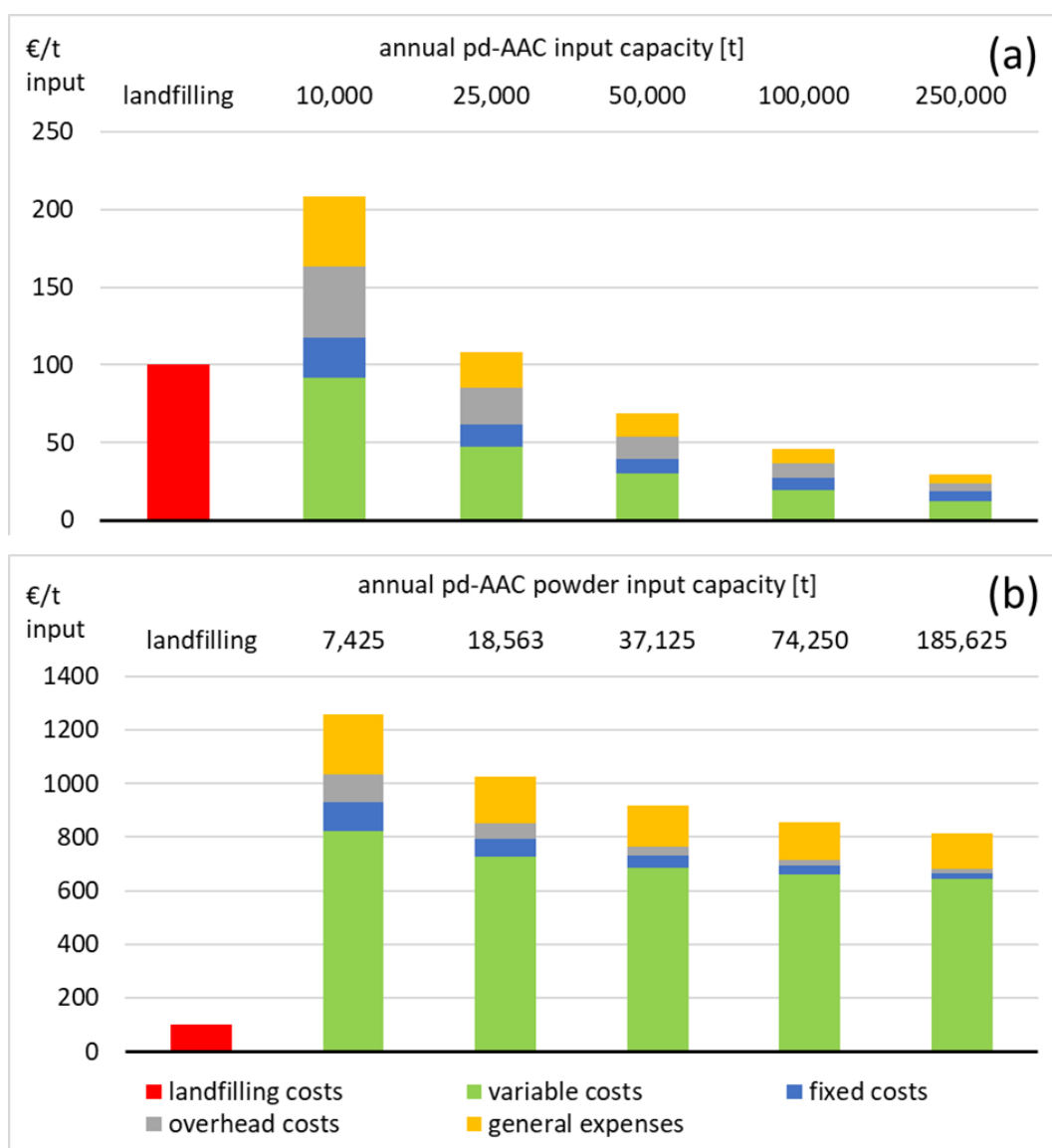
Figure E.2: Total costs of mechanical pd-AAC processing (a) and RC-BCC production (b) and their composition for all considered recycling plant capacities.
