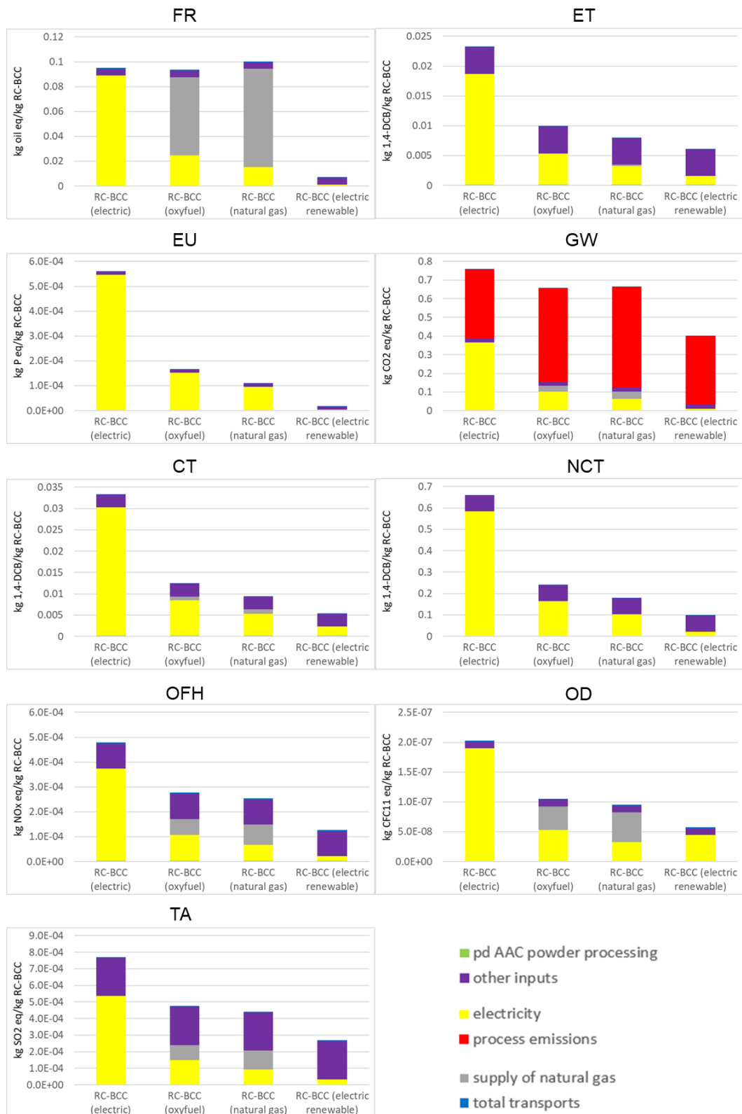
Figure 4.11: LCA results for RC-BCC production with different firing conditions including the midpoints Fossil resource scarcity (FR), Freshwater ecotoxicity (ET), Freshwater eutrophication (EU), Global warming (GW), Human carcinogenic toxicity (CT), Human non-carcinogenic toxicity (NCT), Ozone formation – Human health (OFH), Stratospheric ozone depletion (OD), and Terrestrial acidification (TA).
