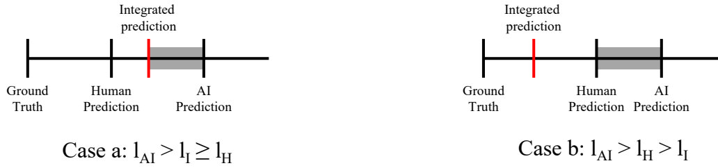
Figure 5.2.: Deviation of human prediction, AI prediction and integrated prediction from the ground truth for a single instance. Possible cases of how realized inherent complementarity potential CP_{theoretical}^{inh} emerges, considering the scenario L_{AI} < L_H
