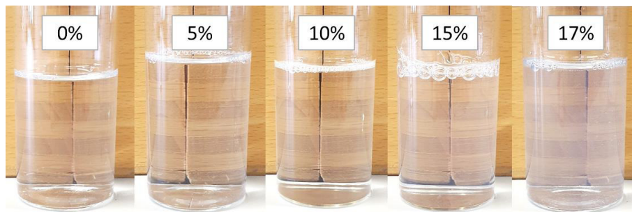
Figure 4-8 Comparison of the four outer water phases used plus another two percent polyvinyl alcohol solution with 17% ammonium chloride. No turbidity can be seen between 0% and 10%. At 15%, a very weak turbidity can be seen, which is more pronounced at 17%.
