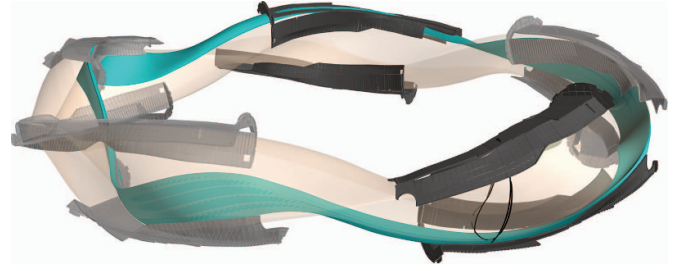
Figure 1. A 3D visualization of the W7-X target geometry. One of the five total islands is plotted in blue. This island intersects the divertor targets in two toroidal modules. These modules are plotted in darker colors as compared to the other toroidal modules. The island intersects the lower target, plotted in dark gray, in the module at the front of the image and the upper divertor in the module in the back of the image. A poloidal slice of the island and the last closed flux surface is plotted in black at toroidal angle \varphi = -10^\circ .
