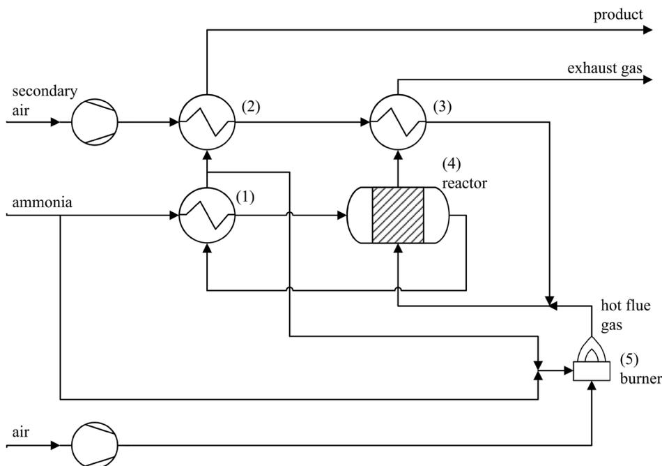
**Figure 2.** Simplified process flow diagram of the ammonia cracker.
