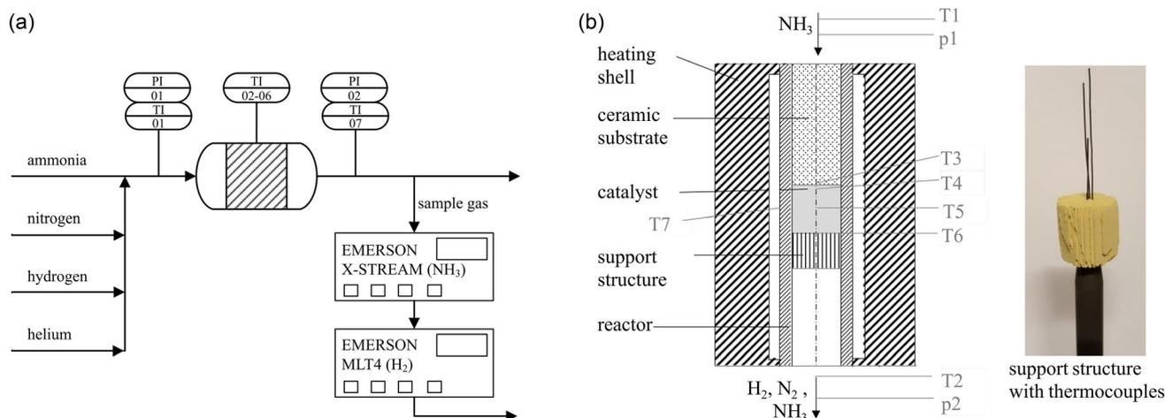
**Figure 3.** a) Simplified flow diagram of the test rig for catalyst characterization and b) cross section of the integral reactor.
