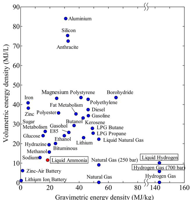
**Figure 4.** Gravimetric and volumetric energy density of combustible materials and batteries according to ref. [67].
