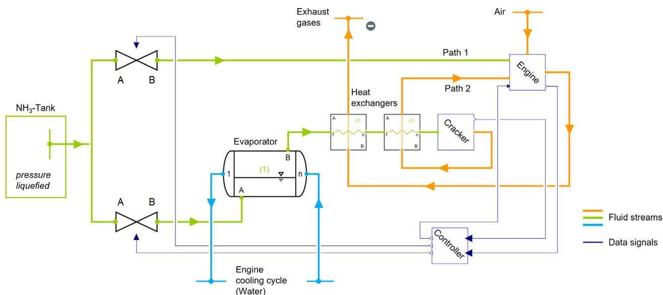
**Figure 12.** Model of the system integration (simulation software: Dymola).
