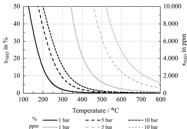
**Figure 1.** Simulated equilibrium ammonia mole fraction as a function of temperature at a pressure of 1, 5, and 10 bar, simulated with Aspen Plus.
