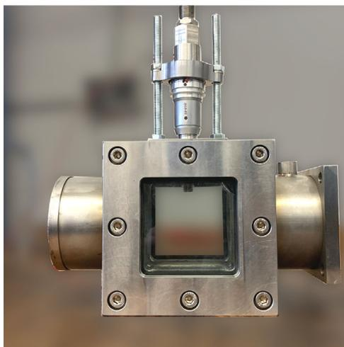
**Figure 9.** Optical intake manifold.
