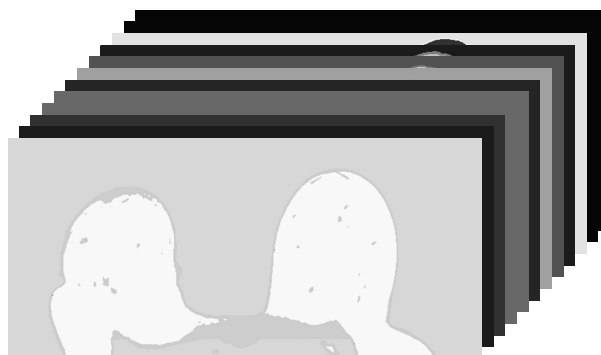
Figure 7.6: An example of one dataset that is segmented by 2D stacked volume. Each slice has different labels than the slice before or after.
