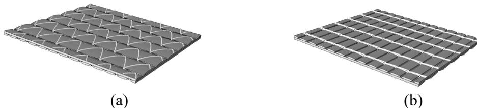
Fig. 2. Geometrical model of biaxial NCF (a) warp yarn view (b) weft yarn view
