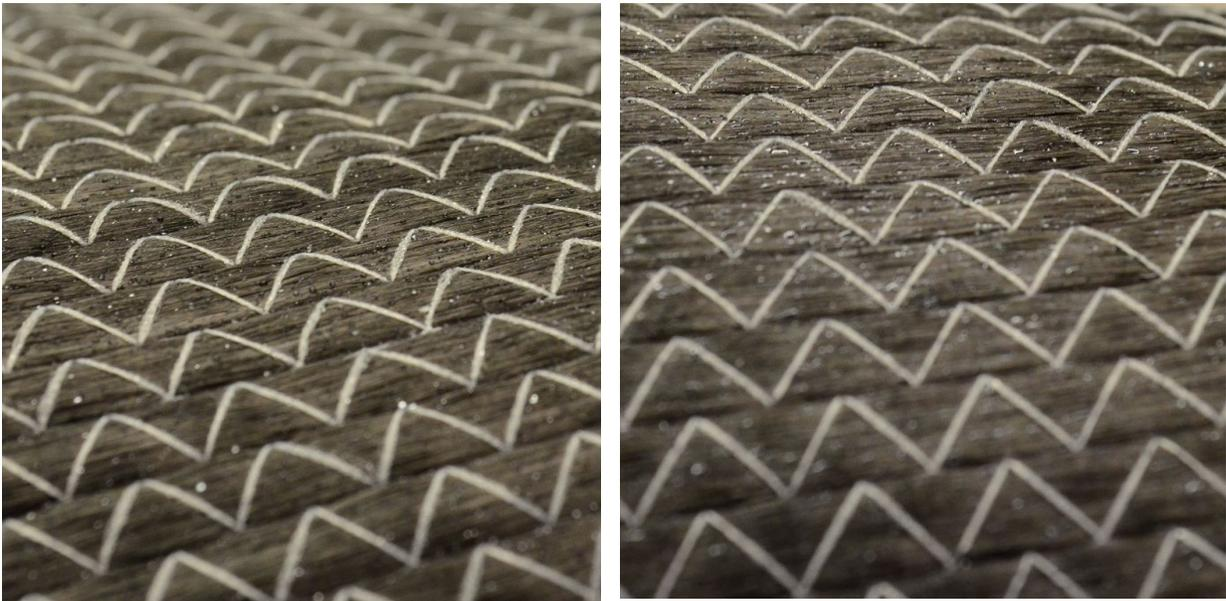
Figure 6: Binder-stabilized UD-NCF; left: Inactivated binder; right: Pre-activated binder in the oven at 120°C.
