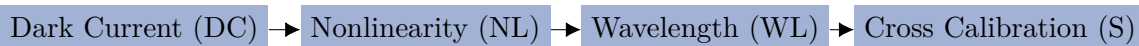
Figure (4.4) The calibration process aims to individually characterize the sensors (DC, NL, WL) and to calculate the cross calibration factor (S) between them. The cross calibrated sensors enable the direct measurement of the remote sensing ratio.
