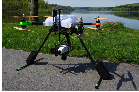
Figure (4.2) Integrated sensor system mounted to the UAV. The two axis gimbal maintains the desired viewing angle of the cameras during the flight. The irradiance spectrometer is mounted on a pole next to the GPS antenna.
