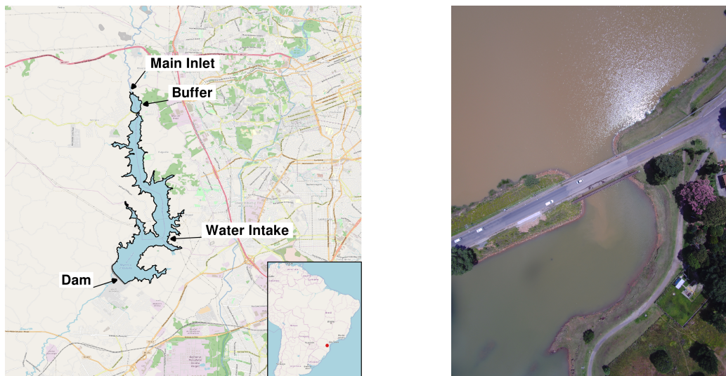
Figure (5.1) Passaúna reservoir, located in the west of Cuitiba, Brazil. The right image shows an RGB image acquired with the system. It shows the area where the water passes the bridge at the end of the buffer. In the upper part of the image, the water of the buffer with a high sediment concentration can be seen, and a gradient after passing the bridge. Map data ©OpenStreetMap contributors.
