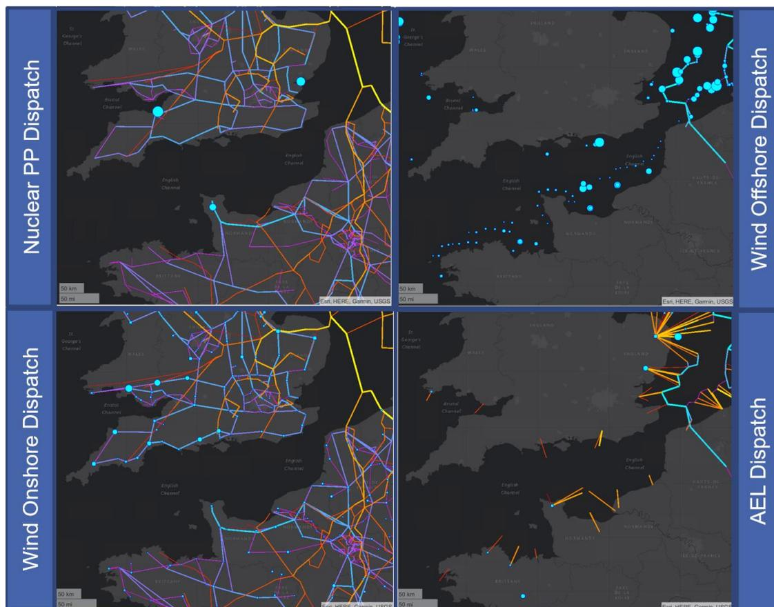
Figure A.27: Comparison of the cumulated dispatch of electrolyzers (bottom right), wind offshore units (top, right), wind onshore units (bottom left) and nuclear power plants (top left) in the English Channel region in 2050
