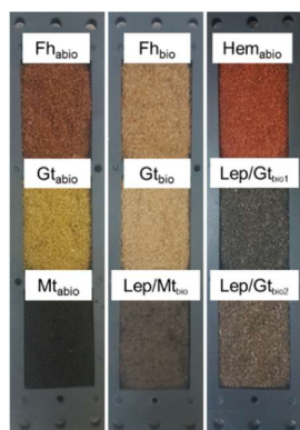
Figure 21: Incubation setup showing the various biotic (bio) and abiotic (abio) mineral coatings in the characteristic mineral colours before the experiment
