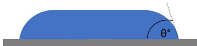
Figure 1.4: Drop with a volume larger than its capillary length and thus flattened contour on a surface.
