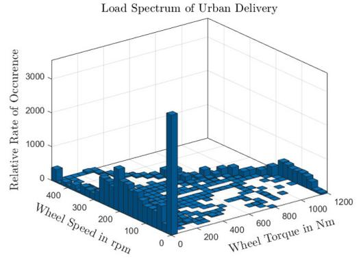
Fig. 5: Visualization of the load spectrum calculated with the Urban-Delivery drive cycle with a 30 kW-map and a total ratio of  $i_{w,\text{ideal}} = 26.3$ , or approximately  $13\,000 \text{ min}^{-1}$  at the generator side.
