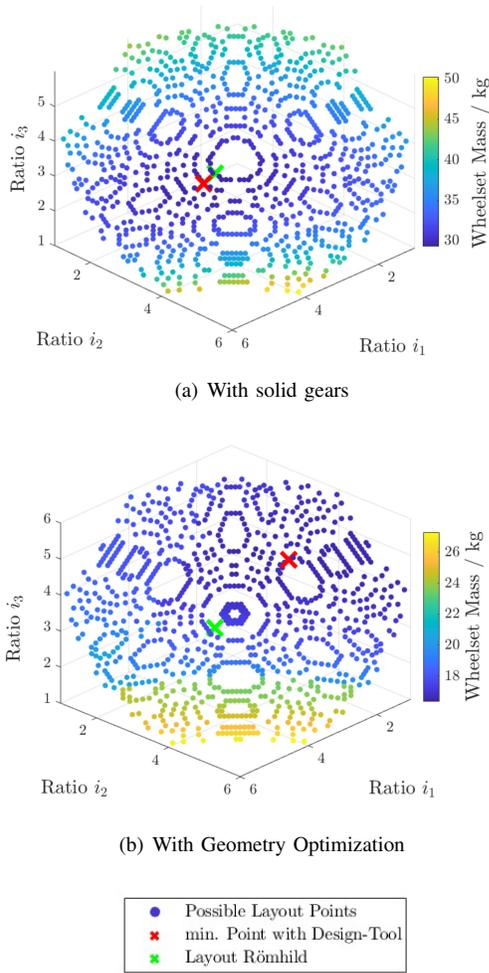
Fig. 6: Comparison of the ideal gear ratio distribution according to the developed design tool and Römhild [10] for three-stage spur gears for minimum wheelset mass, with solid gears and geometry optimization according to Wittel [11].
