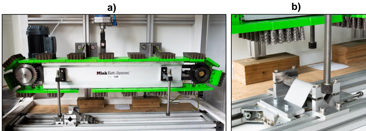
Figure 5-2: a) Abrasion apparatus. b) Clamped filter medium sample.
