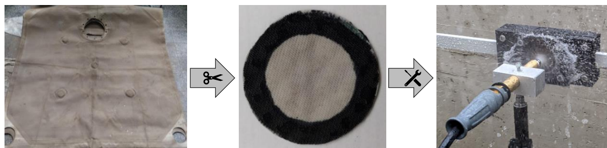
Figure 6-2: Methodology of permeability test samples preparation including jet cleaning.
