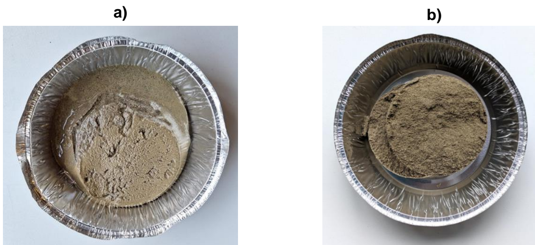
Figure 4-21: Example of two 40 mm filter cakes: (a) 250 kPa filtration pressure, no air blow, average water content 20.2 w%, saturation 100 v%, average shear adhesion 0.9 \text{ kN m}^{-2} , average shear cohesion 1.2 \text{ kN m}^{-2} ; (b) 1250 kPa filtration pressure, 180 s air blow, 550 kPa air blow pressure, average water content 15.7 w%, average saturation 75 v%, average shear adhesion 3.1 \text{ kN m}^{-2} , average shear cohesion 5.0 \text{ kN m}^{-2} .
