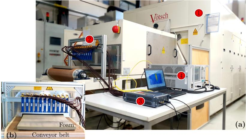
Fig. 3.1: (a) MWT system and its integration with the HEPHAISTOS (number Tag 1) is shown. The number Tags 2, 3, and 4 shows the MWT system, Solid state switch, and VNA respectively. (b) shows the enlarged view of the MWT sensor array of X-band open-ended waveguide antennas. Note here only 7 antennas are used in the measurement with the polymer foam.
