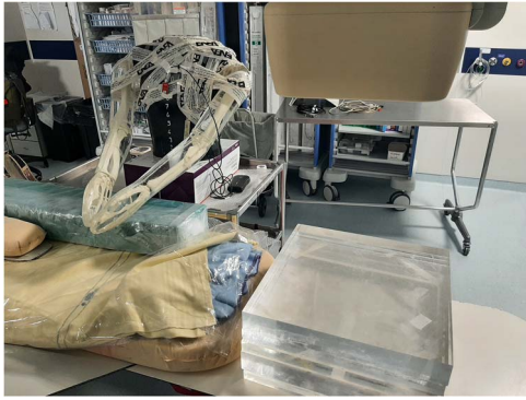
Figure 2. The anthropomorphic thorax phantom representing the operator, with both arms inserted, and the slab transparent phantom representing the patient on the couch.
