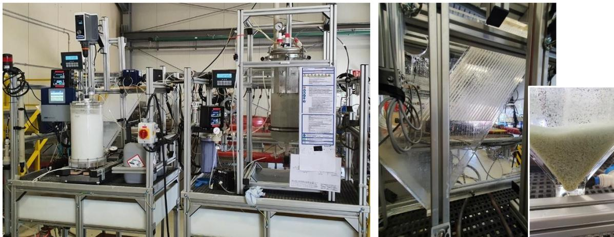
Figure 47: Prototype installed at the geothermal power plant Insheim. The left picture shows the prototype. Precipitates are shown in the two pictures on the right. (Source: Valentin Goldberg / Sebastian Held).
