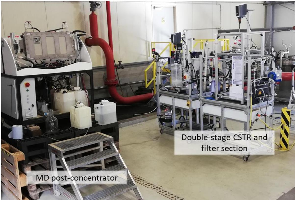
Figure 34: Demonstration plant operated with natural geothermal fluids on-site at power plant Insheim, Upper Rhine Graben, Germany
