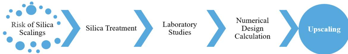
Figure 44: Flow chart summarizing the problem-solving approach in the BrineMine project. Based on the challenge of silica fouling, a treatment strategy was developed in the laboratory. This approach was upscaled first using a numerical design calculation. The simulation results were subsequently reproduced in a technical center leading to the construction of a 1<sup>st</sup> generation prototype.
