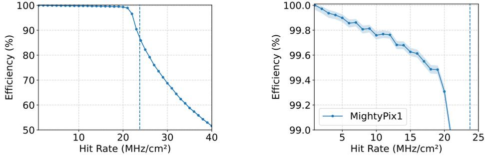
**Figure 2.** Simulated efficiency of the MightyPix1 readout mechanism for hit rates up to 40 MHz/cm<sup>2</sup> (*left*) and a close up of the region with over 99% efficiency (*right*). The CI is shown as blue band, but too narrow to be visible for higher rates. The dashed line at 23.75 MHz/cm<sup>2</sup> marks the readout limit.
