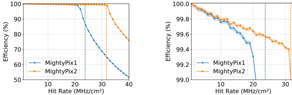
**Figure 5.** Simulated MightyPix2 efficiency for hit rates up to 40 MHz/cm<sup>2</sup> (*left*) and a close up of the region with over 99 % efficiency (*right*). The CIs are shown as blue and orange bands, but too narrow to be visible for higher rates. The dashed lines at 23.75 MHz/cm<sup>2</sup> and 31.66 MHz/cm<sup>2</sup> mark the readout limits.
