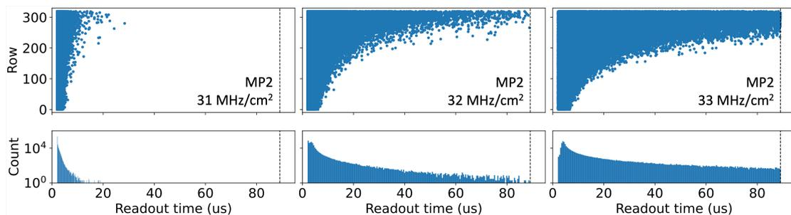
**Figure 6.** Readout time of simulated hits for the 320 rows of MightyPix2 for a hit rate of 31 MHz (*left*), 32 MHz (*middle*), and 33 MHz (*right*). The dashed line at 89.1 μs marks the readout time limit.
