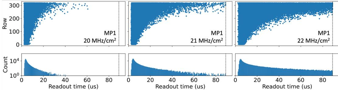
**Figure 3.** Readout time of simulated hits for the 320 rows of MightyPix1 for a hit rate of 20 MHz (*left*), 21 MHz (*middle*), and 22 MHz (*right*). The dashed line at 89.1 μs marks the readout time limit.
