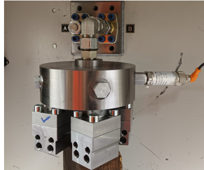
(b) Picture of the mounted test assembly inside the test chamber of the hydraulic test rig.
