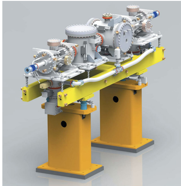
Fig. 199 CAD rendering of the XGM used at the European XFEL. Figure from [267]
