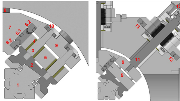
Fig. 172 Cross-section at radial piston (left) and at radial acting rod axis depth (right)
