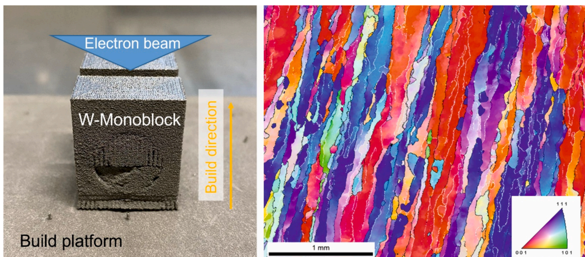
Fig. 9. Microstructure along the building direction. Crystallographic direction parallel to the building direction.
