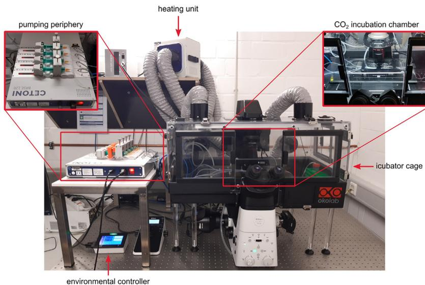
**Figure 2. Experimental setup for a MSCC consisting of an automated live-cell imaging microscope as well as the respective pumping periphery and environmental control**
