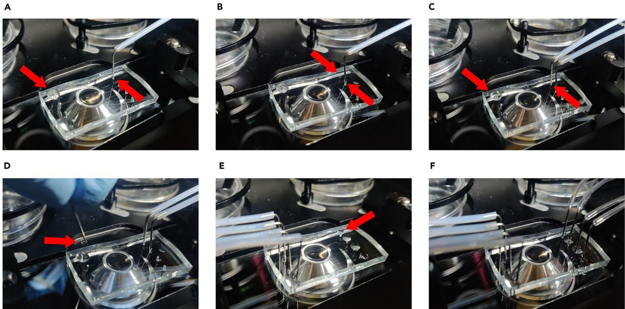
**Figure 6. Inoculation of the microfluidic cultivation device and subsequent establishment of constant perfusion**
