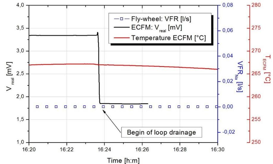
Signals during loop drainage
