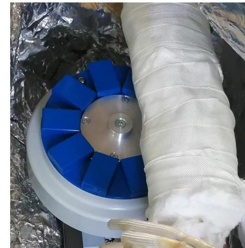
Fly-wheel integrated in SOLTEC-2
