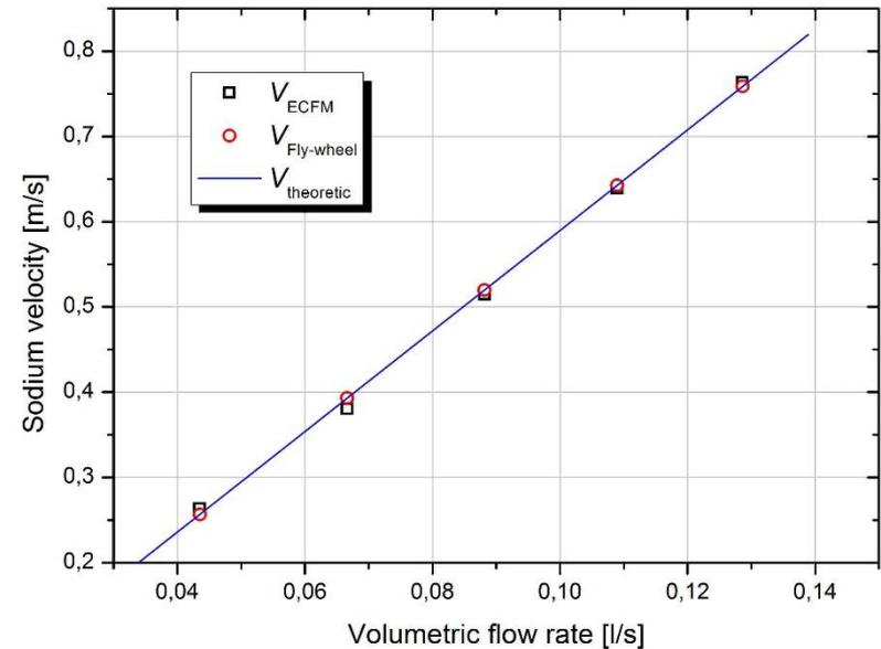
Calibration equation for the ECFM sensor:
