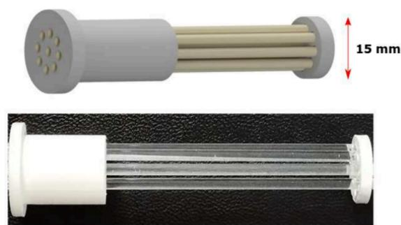
**Figure 2.** Sample holder assembly, 3D-printed using PLA. Nine individual sample capillaries, each with an OD of 2.4 mm, and filled with a sample volume of 150–200  $\mu\text{L}$ , were thus accommodated.
