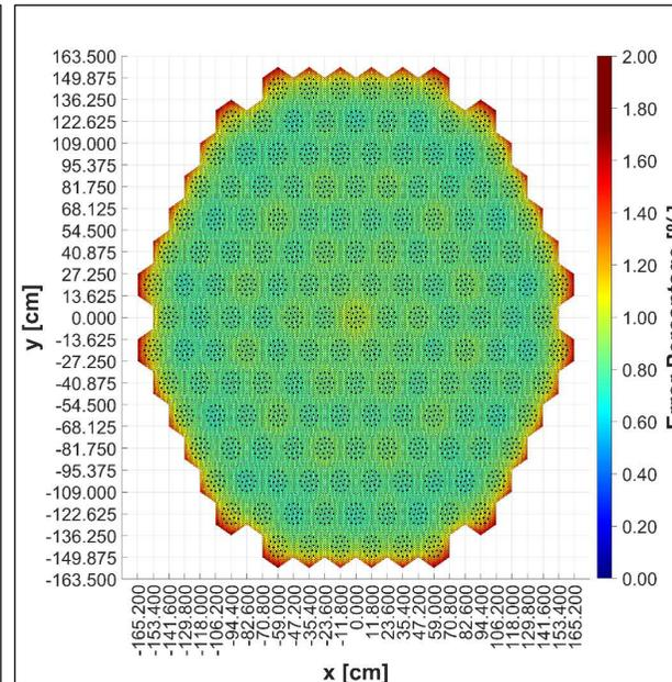
Pin power statistical error distribution in the core
