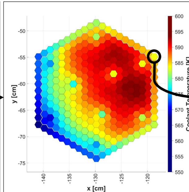
Sub-channel level coolant exit temperature distribution in the FA No. 37 which has the hottest fuel rod center temperature
