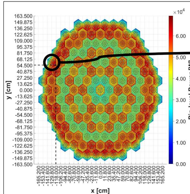
Pin-level power distribution in the core with the location of the fuel with the highest power (similar statistical error distribution trend with previous graph up to 2%)
