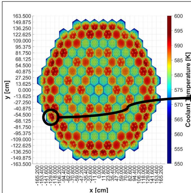
Sub-channel level coolant exit temperature distribution in the core
