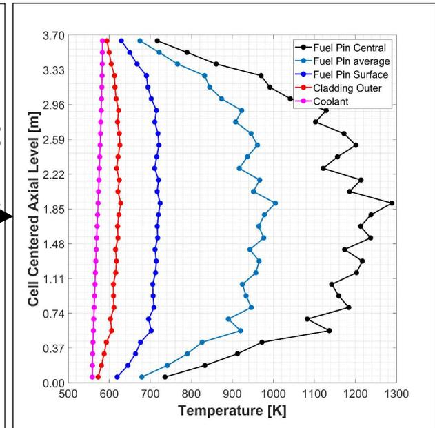
Pin 12247 axial temperature distribution (the hottest fuel rod center temperature in the core)
