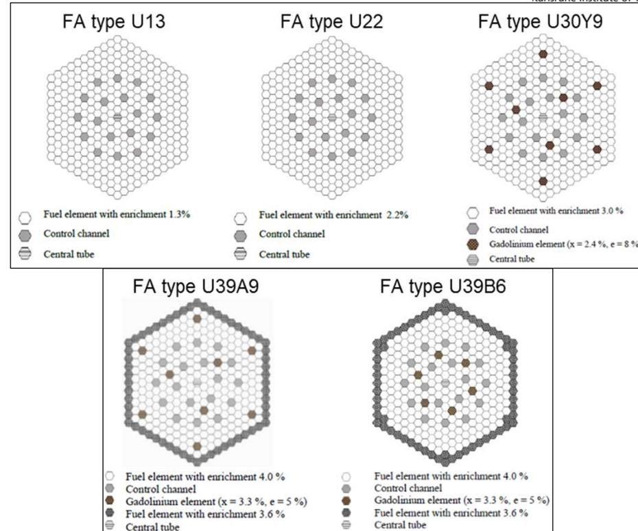
Radial arrangement of elements in the fuel assemblies
