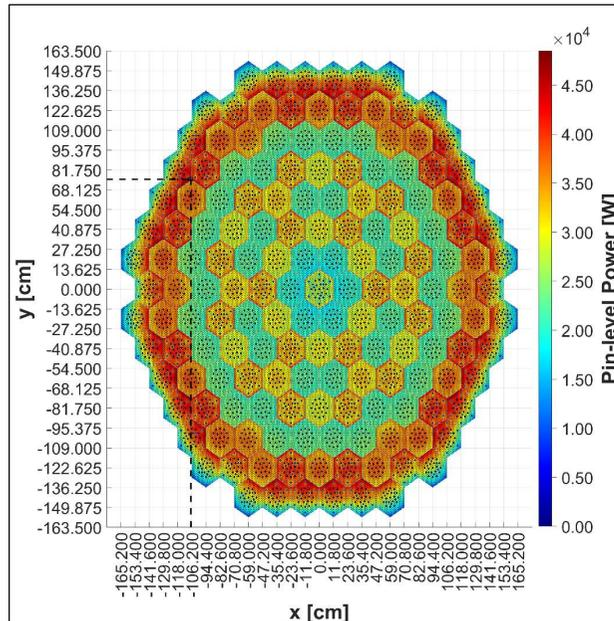
Pin-level power distribution in the core with the location of the pin with the highest power
