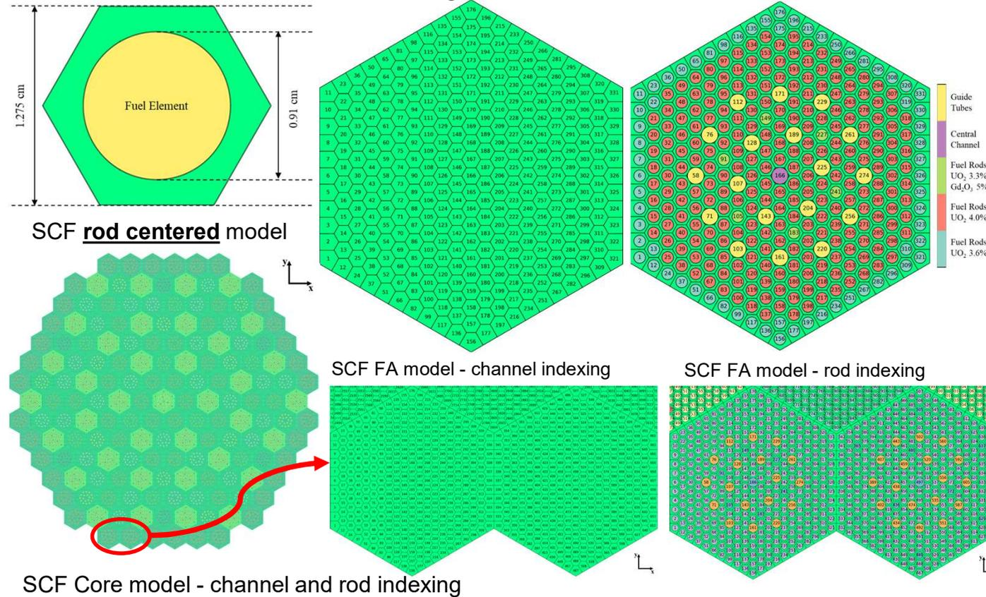
➤ Python based preprocessor was used to generate rod and channel layout and connectivity relations and "ifc" files for code feedback exchange.
