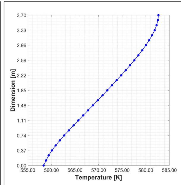
Core average axial coolant temperature distribution
