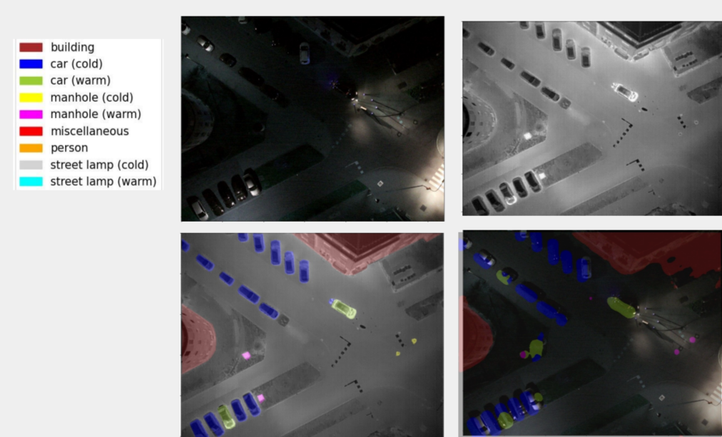
Example of thermal urban feature segmentation (I): combined RGB (top left) and TIR (top right) inputs, manual segmentation mask (bottom left), and U-Net model prediction (bottom right). Source [3]
