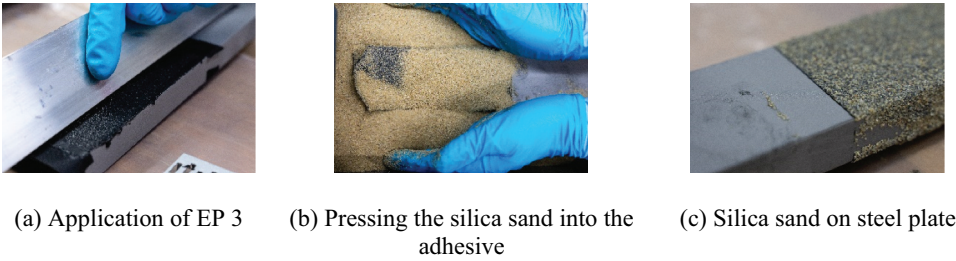
Figure 5. Manufacture of coated surface with silica sand.
