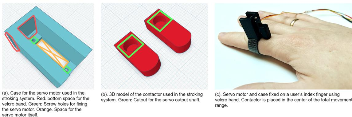
Figure 5.6: 3D models for the case and the contactor, and the implementation on an user's finger of one element of the stroking system.
