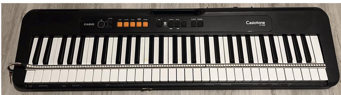
Figure 5.10: Keyboard with attached LED strip with the connector of the LED strip on the left side.
