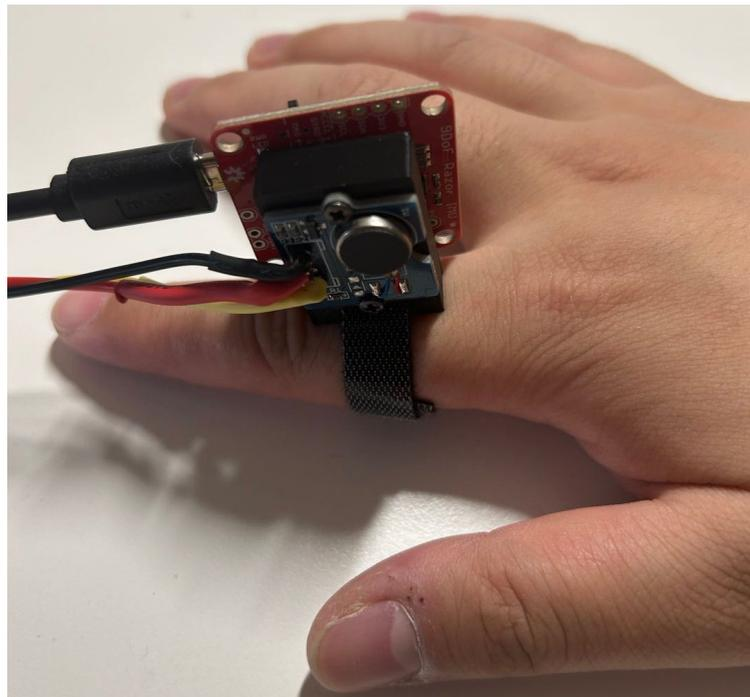
Figure 5.7: Experiment setup: An accelerometer is mounted on the back side of the vibration actuator.
