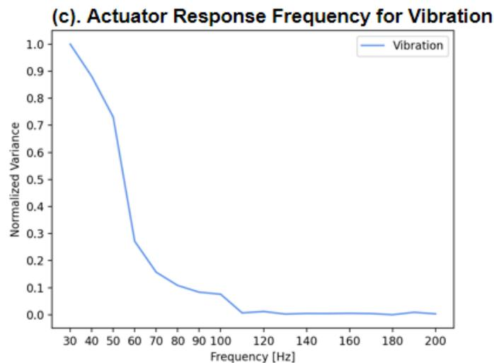
Figure 4.10: Evaluation results for actuator response frequency for vibration.
