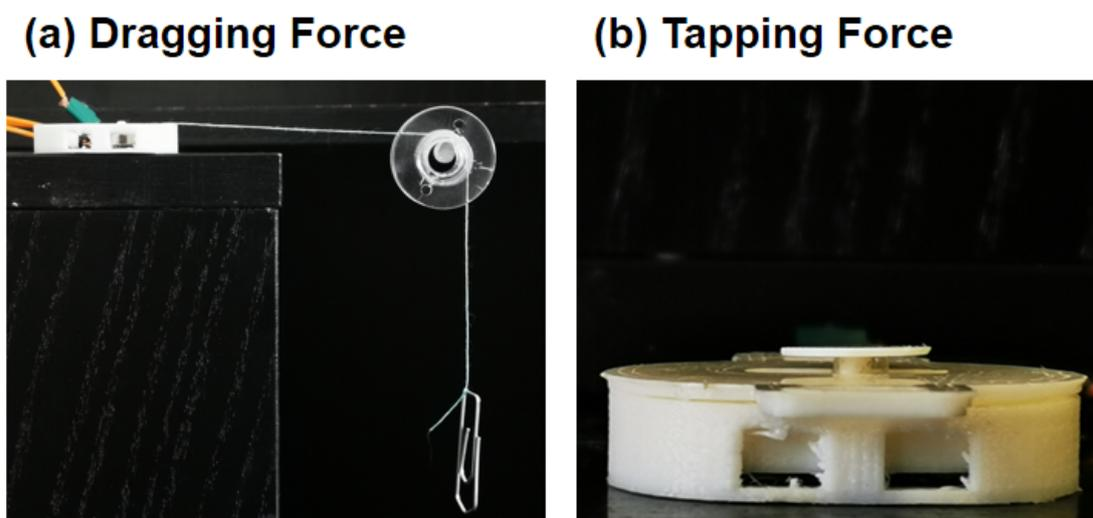
Figure 4.8: Force test setup: (a). dragging; (b). tapping.
