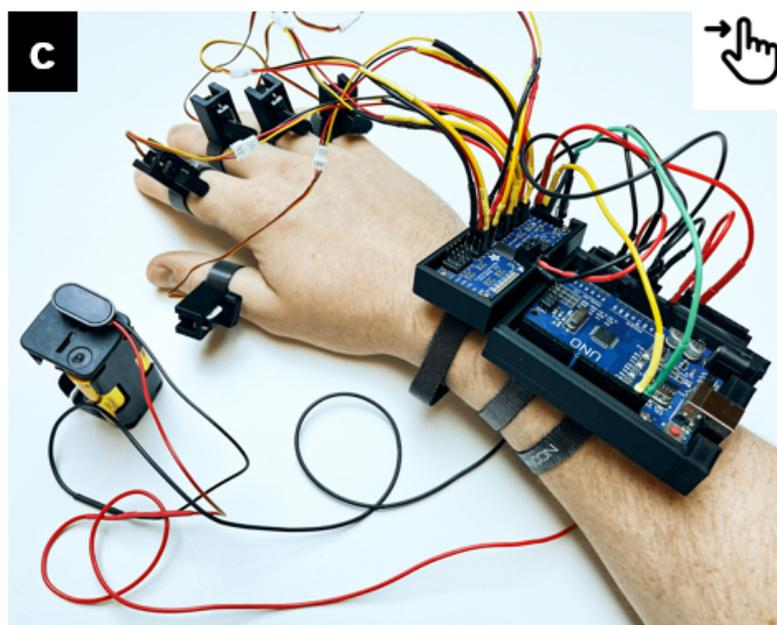
Figure 5.3: Stroking system attached to an user's forearm.
