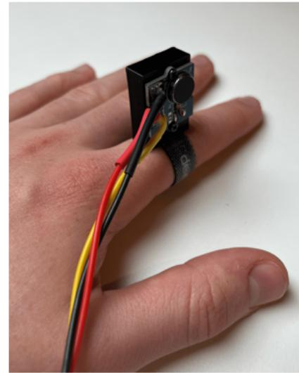
(b). Vibration motor and case fixed on the index finger of a user using a velcro band.
