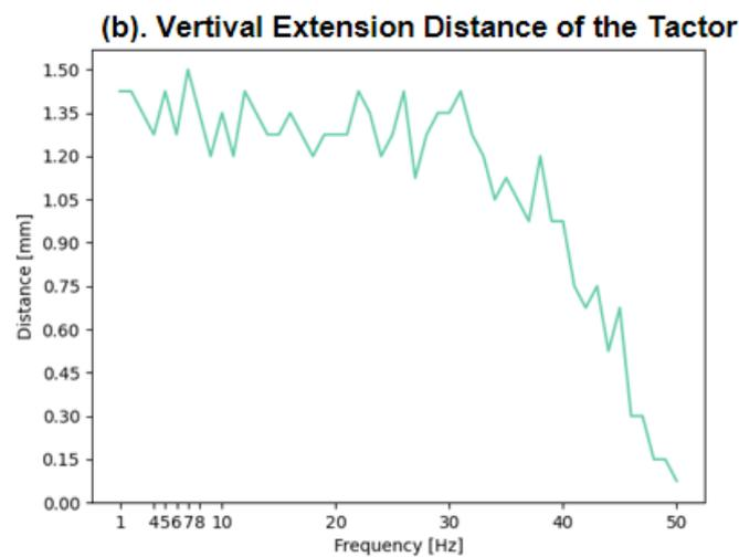
Figure 4.9: Evaluation results for vertical extension distance of the tactor.
