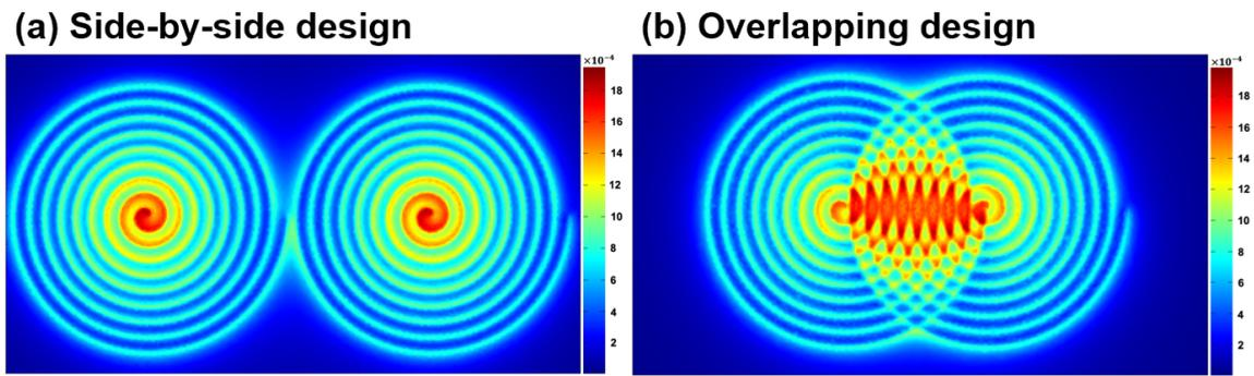
Figure 4.5: Simulation of the magnetic field: (a). side-by-side coil design; (b). overlapping coil design.
