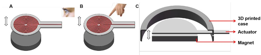
Figure 3.7: (A). *Observe*; (B). *Hover*; (C). Section view of 3D printed case to place the finger used in the *Rest* scenario.
