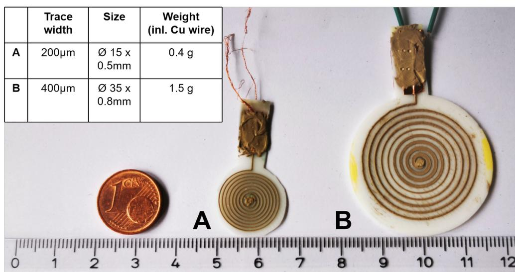
Figure 3.4: Various diameters and trace width/distance configurations.
