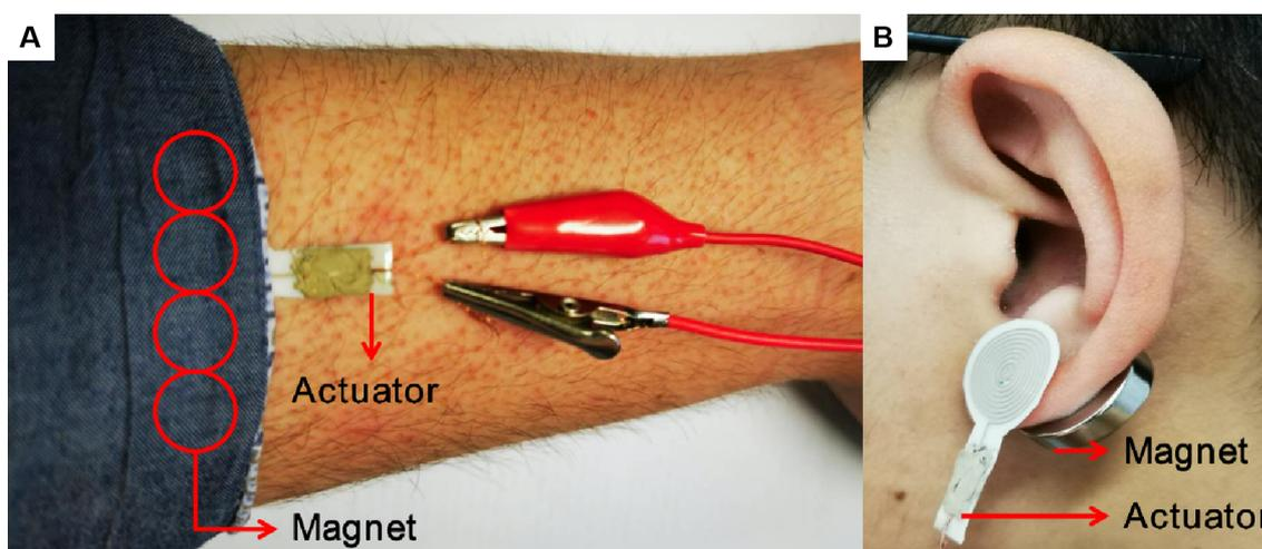
Figure 3.8: Application: (A). Vibration sleeves; (B). Earring-shaped haptic feedback system.
