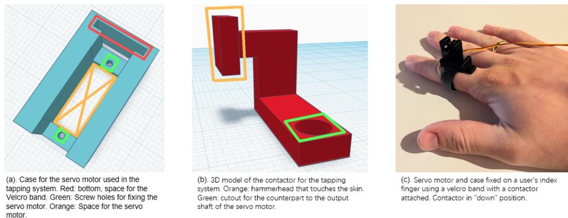
Figure 5.5: 3D models for the case and hammer-shaped contactor, and the implementation on an user's finger of one element of the tapping system.
