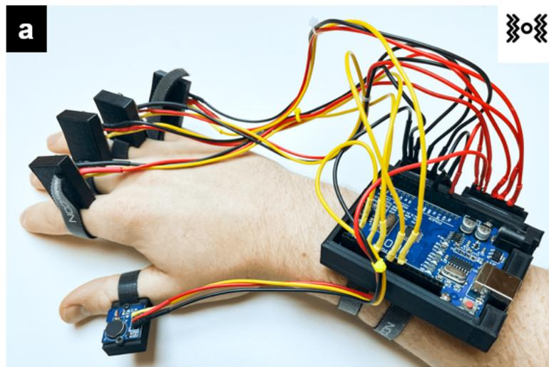
Figure 5.1: Vibration system attached to an user's forearm.
