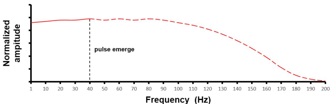
Figure 3.5: Experiment 1 results, Actuator response frequency: 1-200Hz.
