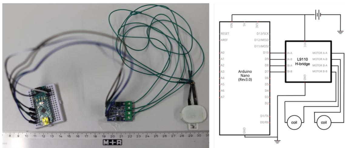
Figure 4.4: Electronics schematic of the USB version actuator.
