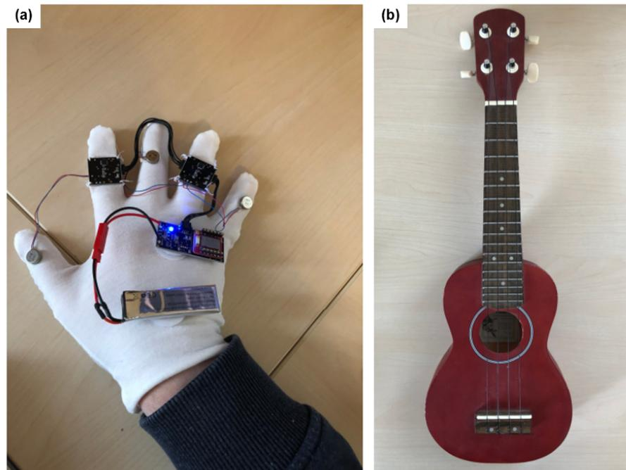
Figure 6.1: Passive Haptic Learning glove and Ukulele: (a). Glove and electronics position on the hand; (b) Ukulele used in the experiment.
