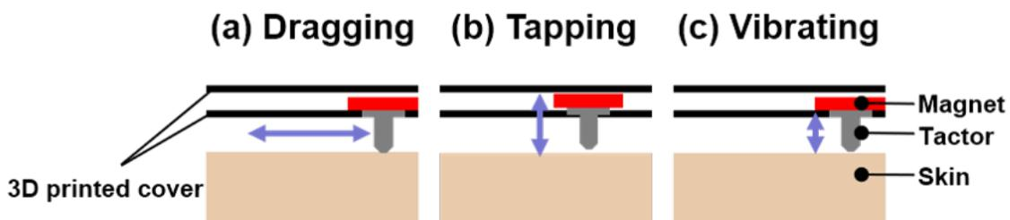
Figure 4.6: Schematic cross-section of the motions of the tactor: (a). dragging; (b). tapping; (c). vibrating.
