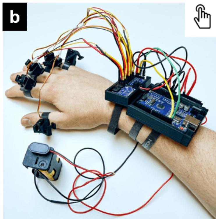
Figure 5.2: Tapping system attached to an user's forearm.
