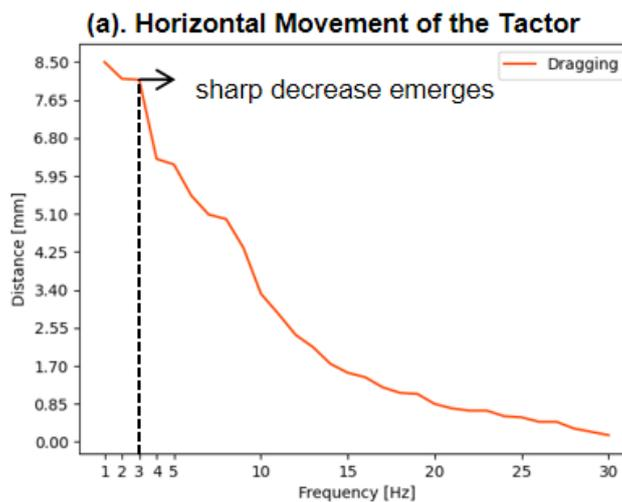
Figure 4.7: Evaluation results for the horizontal movements of the tactor.
