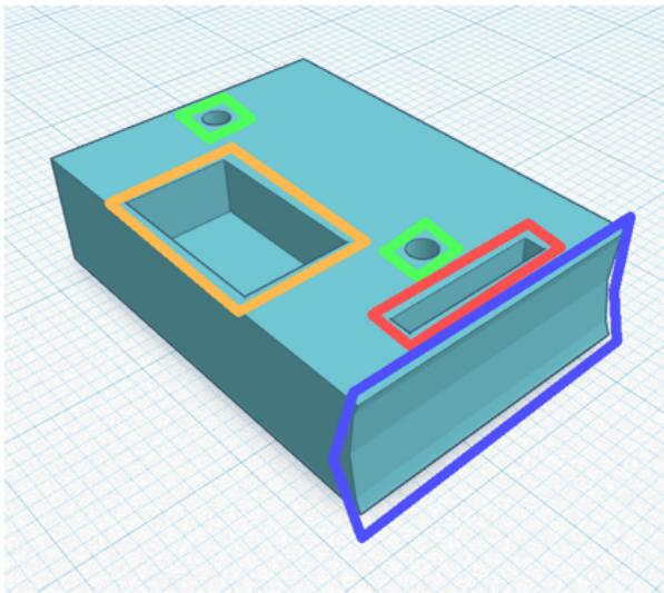
(a). Case for the vibration motor used in the vibration system. Red: bottom, space for the velcro bands. Green: Screw holes for fixing the vibration motor. Orange: Space for the back end of the pins. Blue: curved bottom as a contact to finger.
