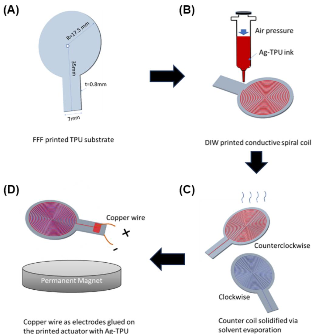
Figure 3.3: The fabrication process involves the following sequential steps: (A). Printing a TPU substrate with a centrally located all-through hole measuring 1mm in diameter; (B). Printing capillary Ag-TPU ink traces on both sides of the substrate; (C). Curing the printed traces to enhance their conductivity and durability; (D). Connecting copper wires and traces using the same Ag-TPU ink to establish electrical connections.
