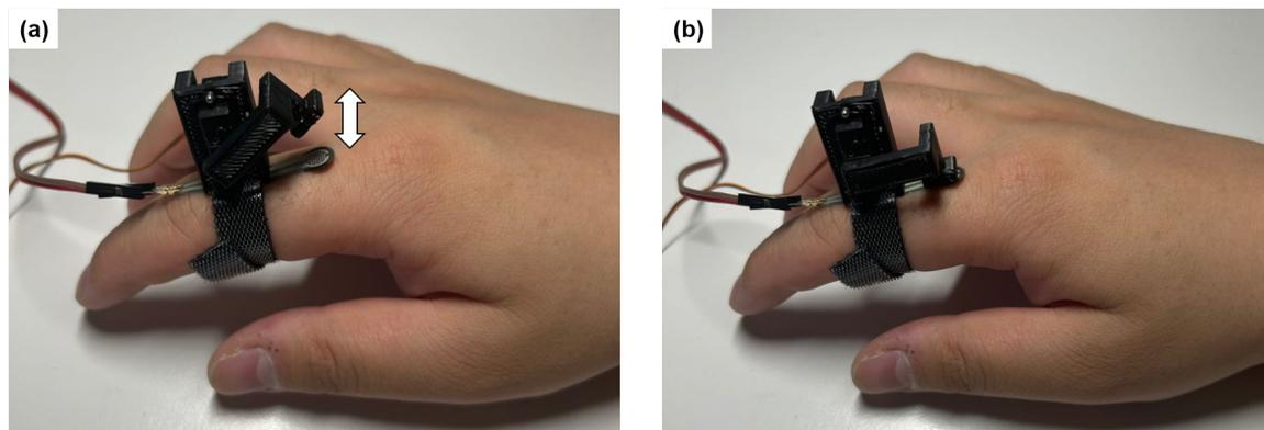
Figure 5.8: The tapping actuator pushes against the user's finger. (a). The contactor lifts up; (b). The contactor falls.
