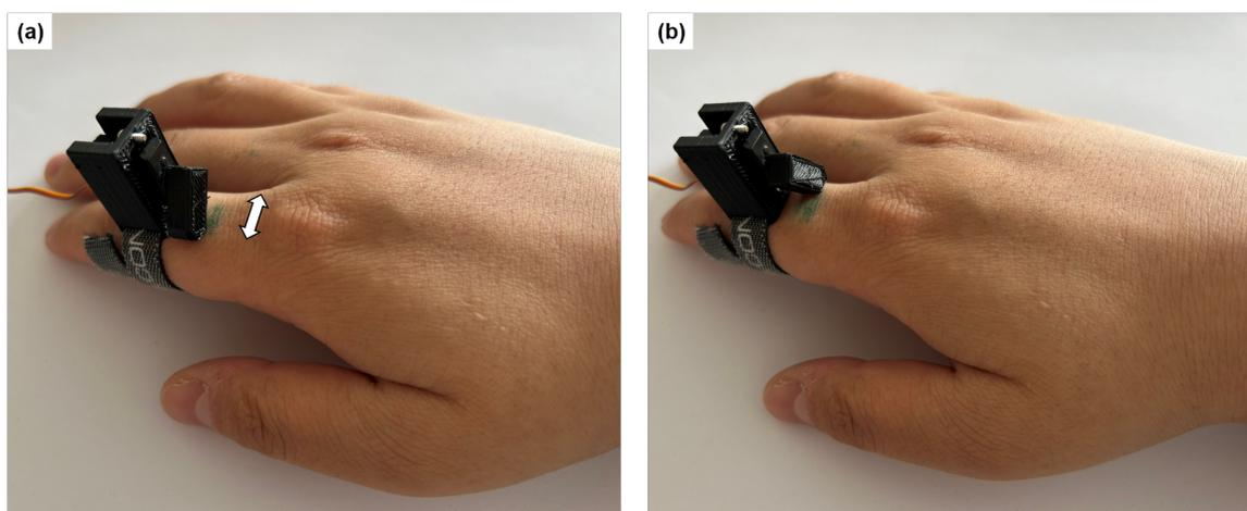
Figure 5.9: The stroking distance of the actuator on the hand. The green ink shows the result of a contact test. (a). The schematic diagram of the movement of the contactor; (b). The movement distance of the contactor.
