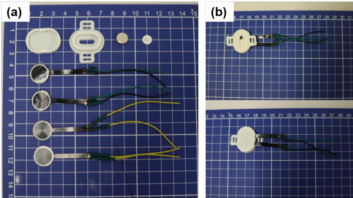
Figure 4.3: *DragTapVib*'s components and assembly. (a). All components before assembly; (b). A completed device.
