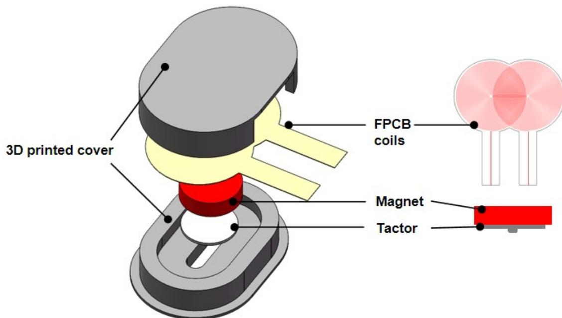
Figure 4.2: Explosion view of the *DragTapVib*.
