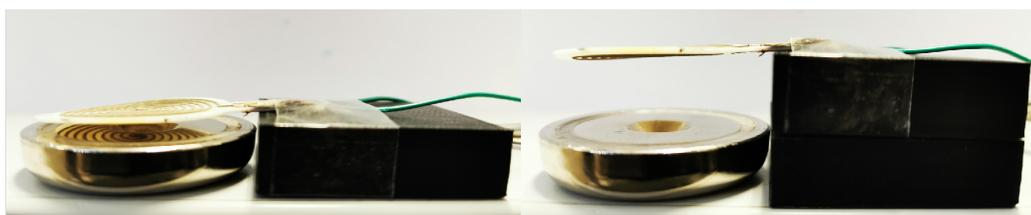
Figure 3.6: Experiment 2 set up: 3D-printed cubes for varying distance.
