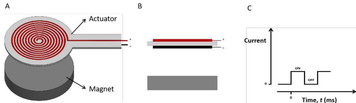
Figure 3.2: (A). 3D view of the *FLECTILE* with printed coils designed in clockwise and counterclockwise on two sides of the substrate; (B). Front view of the placement of *FLECTILE* and the magnet; (C). Utilizing a driving method that involves switching on and off a 5V DC power source.
