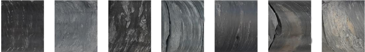
Figure 23: Categories identified on the surfaces of the drill cores BDR-D1 and -D2. From left to right: dark grey clay matrix, turbated light-grey sand/carbonate matrix, light-grey sand/carbonate concretions, light-grey sand/carbonate layers, bituminous lenses (i.e. the small black spot below the middle of the image, embedded in clay matrix), brownish concretions (likely iron-rich (siderite)), fossil-rich layer (containing mussel shell fragments (coquinas) besides brownish concretions).
