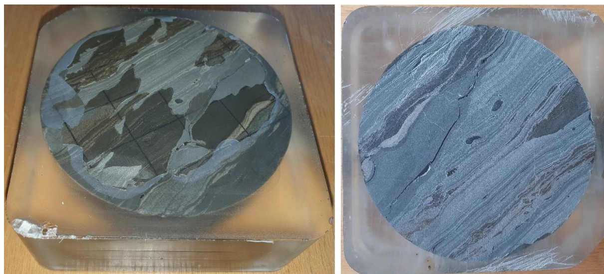
Figure 96: Intact clay rock samples before (left) and after (right) the abrasion of the protruding residue on the surface.
