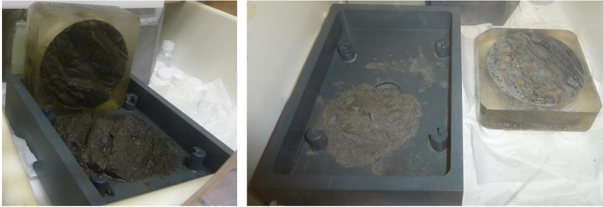
Figure 97: Results of contacting the big rock surface sorption samples with synthetic pore water.
