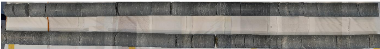
Figure 16: Cores BDR-D1 and -D2, segment 5.0–8.0 m laid next to each other at the same well-depth as a compilation of multiple pictures.
