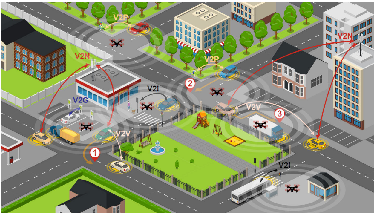
FIGURE 8. Representation of a Jamming swarming attack with several jammers interfering in the V2X communication.
